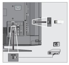
Connect the »USB HDD« socket of the television and the corresponding socket on the data device (external hard drive, digital camera, card reader or MP3 player) using a USB cable;
